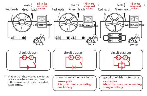
Summarize the relationship between how to connect dry batteries and the strength of the current
