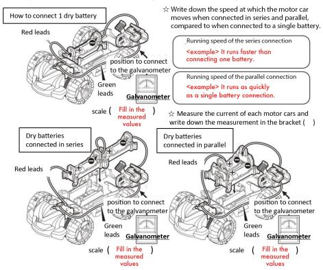
☆ Let's look at each motor car from above and add a circuit diagram to the diagram below.
