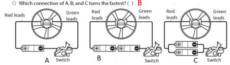
☆ What is the name of the method used to connect the batteries in B and C? Let's write in the brackets ( ) below.
