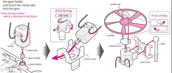
OAttach the motor to the motor cover
