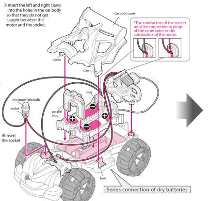
Use manganese dry cell batteries for this teaching material. Alkaline batteries and rechargeable batteries have a large amount of current. If you accidentally connect the + and - terminals of the battery directly, the battery and the conductors may become hot, resulting in burns or a fire. Please read the instructions on the battery carefully before use.
