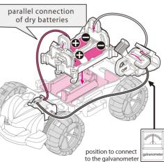
Oremove motor and socket (miniature light bulb), assemble while paying attention to the orientation of the batteries and how to connect the wires.
