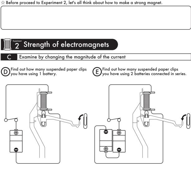
$\gtrsim$  When using a galvanometer in Experiment 2-C, try drawing the schematic symbols in the figure above.
