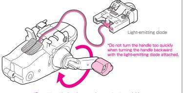
\*Do not turn the hand-powered generator too quickly, It may cause the miniature bulb or light-emitting diode to burn out.
