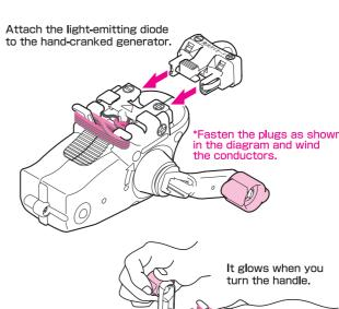
①Turn the capacitor switch off and turn the handle to store the electricity. ②After storing the electricity it glows when the switch is turned on (ON).
