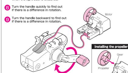
Replace it with a buzzer and turn the handle in the same way.
