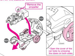
Tighten the car's cover, turn on the capacitor switch. and get it to move.
