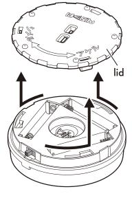
Insert the batteries in the correct direction and close the lid.
